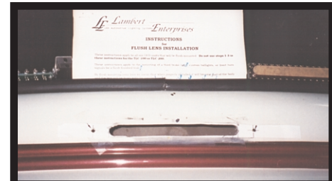
Stud holes drilled & lens opening cut out.
